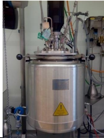
20-L autoclave vessel 150-250°C
